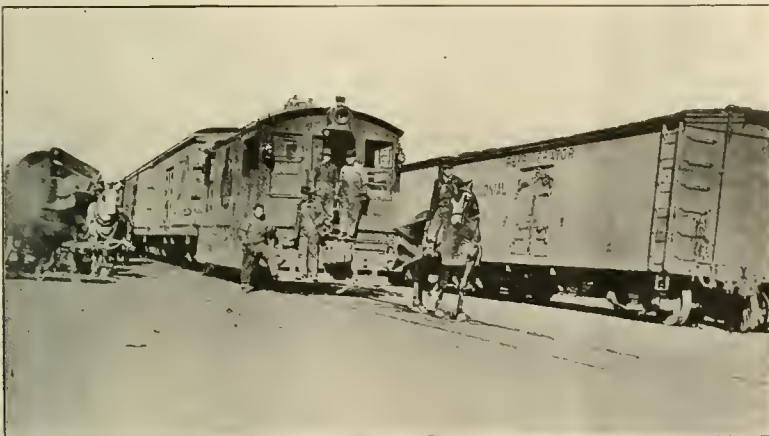
MOUNTED FLAGMAN AND DUMMY ENGINE WAITING AT A CROSS STREET IN NEW YORK.
